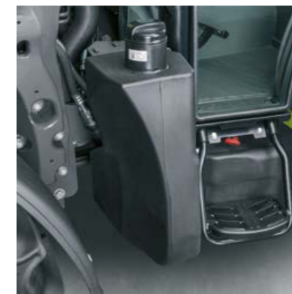
The 95 l diesel tank and the 10 l urea tank provide enough range for long working days
