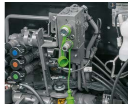
The hydraulic two-line trailer brake enables you to remain flexible during transport operations
