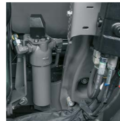
The oil filters in the engine are easy to reach even with a front loader bracket
