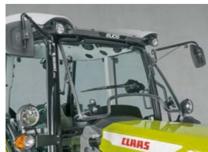
The front windscreen opens for natural ventilation
