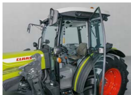
The large doors open wide without protruding too far beyond the sides of the vehicle, enabling you to climb on board easily even in confined spaces in buildings
