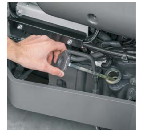
The oil level can be checked and topped up on the right-hand side of the ELIOS 200 when the bonnet is closed
