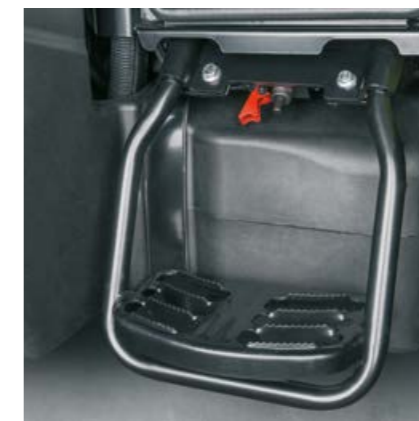
The battery isolating switch is conveniently located on the left access step (except ELIOS 210)
