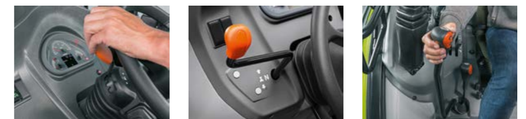
The reverser for mechanical reversing and the electronic REVERSHIFT are handily positioned to the left of the steering wheel
