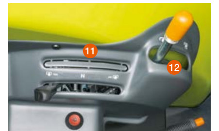
The PTO is engaged with hydraulic support as standard. Electronic PTO engagement is available as an option in machines with REVERSHIFT.
