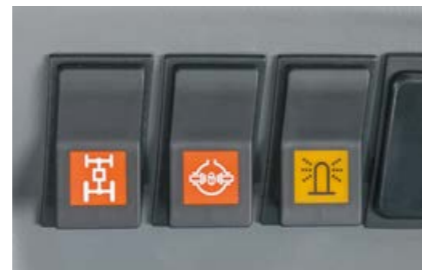
Electrical four-wheel drive and differential lock engagement: the speed-dependent safety cut-out prevents operating errors
