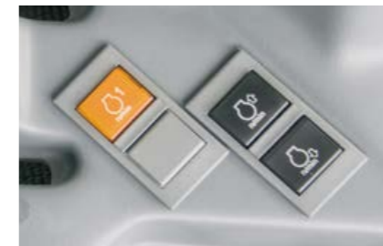
PTO work is very simple with the ELIOS, as the engine-speed memory is part of the standard specification
